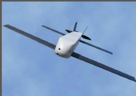
**SWITCHBLADE** – Rapid Response - Precision Strike - Low Collateral Damage. A low cost, man-portable, lethal micromunition for day/night direct and indirect fire missions. A tube-launched UAS designed with lock-on and forget capabilities is ideally suited for one-soldier operation in the most challenging environments.
